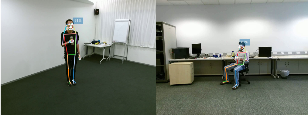
Figure 6.6: Examples of skeletons estimated with OpenPifPaf on the NTU RGB+D dataset.
