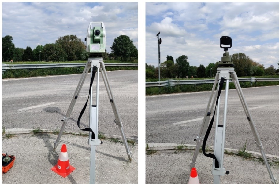
Figure 6.6: Total station and prism target setup
