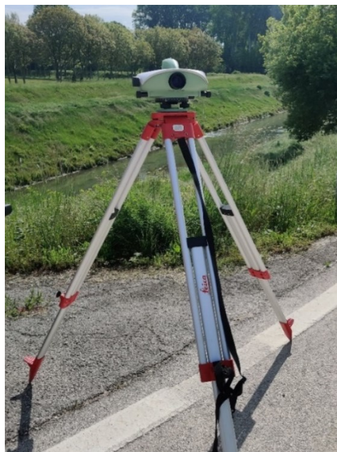
Figure 6.5: Geometric levelling setup
