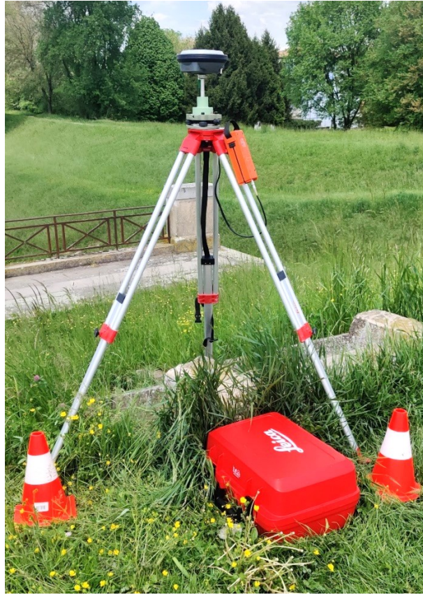
Figure 6.7: RTK GNSS setup
