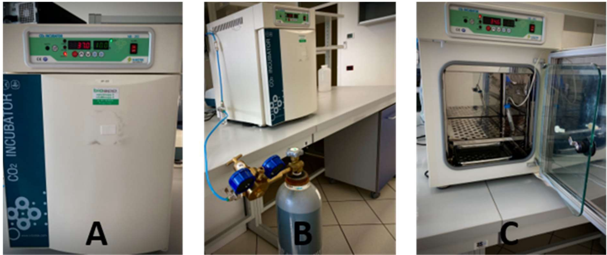
Figure 12: CO 2 incubator setup used. (A) closed incubator with a dashboard for choosing temperature and CO 2 concentration, (B) a CO 2 cylinder connected to the incubator, and (C) an open incubator with shelves on which to place samples.
