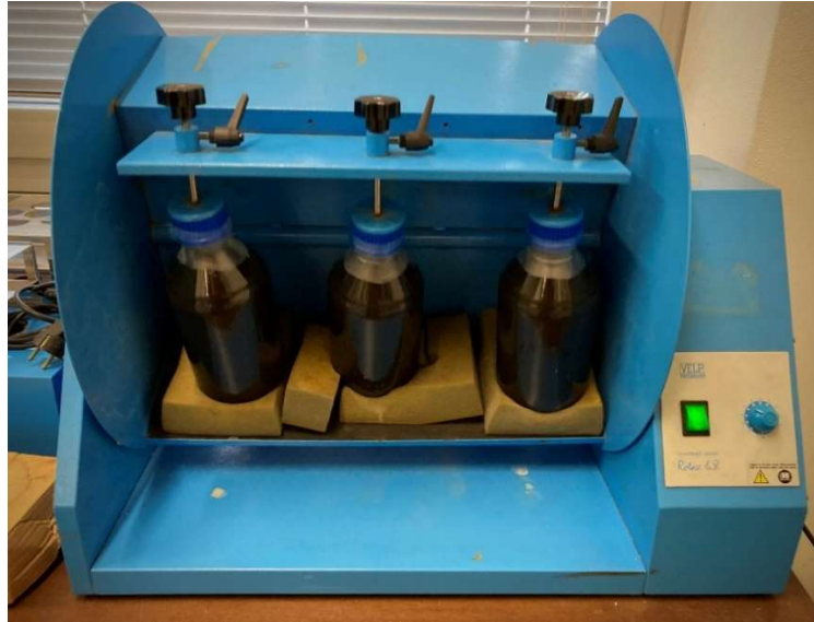
Figure 14: Rotax 6.8 rotary mixer used for the leaching tests.
