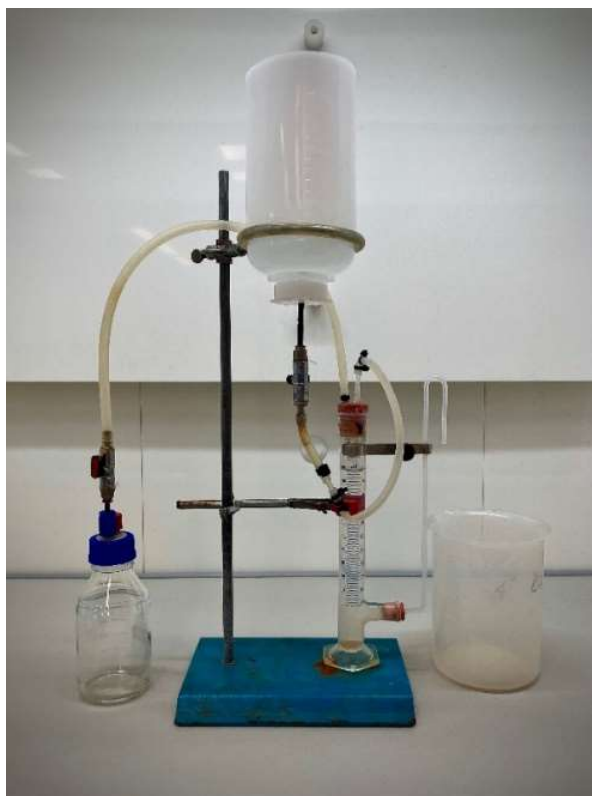
Figure 13: Calcimeter used for the analysis of pre-and post-carbonation materials.
