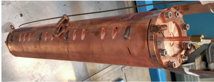
Figure 3.4: Cavity used, showing the aperture into two halves and the return springs
