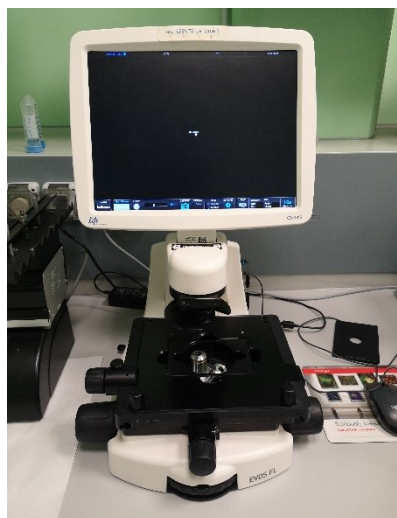
Figure 2.40 Invitrogen EVOSTM FL Cell Imaging System by Thermo Fischer Scientific used in BIAMET Laboratory.
