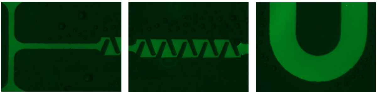
Figure 3.62 Result of the validation experiment with fluorescent isothiocyanate-dextran on the irreversible configuration of the first microfluidic platform.
