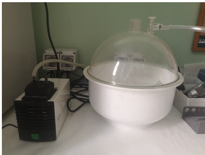
Figure 2.38 Desiccator connected to the vacuum pump used in the BIAMET Laboratory.
