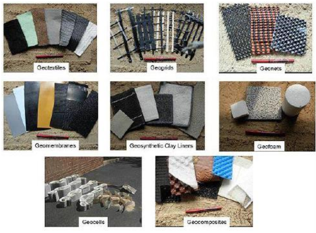
Figure 1.12. Photographs illustrating the various types of geosynthetics (Brezzi, 2019)
