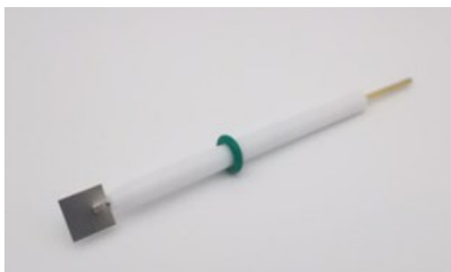
Figure 2.10: Platinum Sheet Electrode
