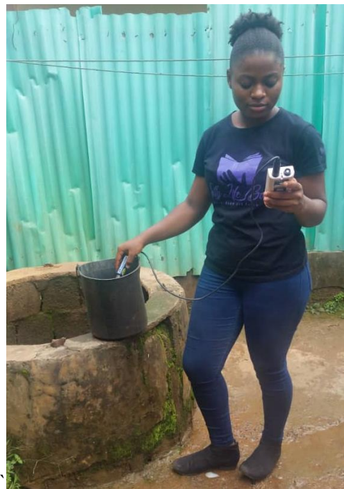
Figure 16: Temperature recording onsite using an ORP meter
