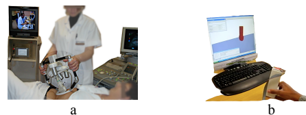
Figure 1: (a) positioning of the light-weight (< 3 kg) Prosit 1 robot on the patient (b) haptic probe held by the expert for the orientation of the remote ultrasound probe holder robot
