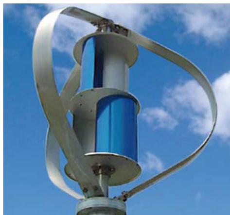
**Figura 2.10** *Turbina Darrieus-Savonius*
