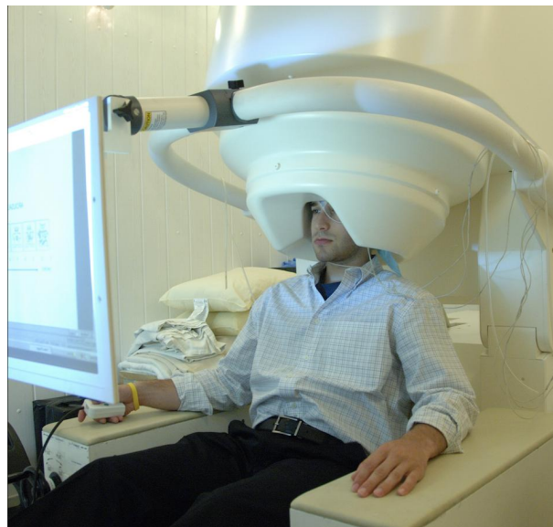
Figure 1.3: MEG structure is set around subject's head: to avoid artifact, the patient should not move his head or do any type of movement of facial muscles. The acquisition is painless and, usually, used with a shielded EEG headset
