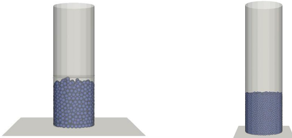
Figure 5.2.a, 5.2.b: Simulation state at the end of the deposition phase, for a 20:1 sample (a) and a 10:1 (b) sample scaling.
