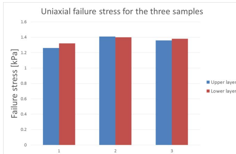
Figure 3.23.b: Uniaxial failure stress for the three batches of MCC Cp-102+30000 cSt silicone oil tested, comparing the results of the upper layer and of the lower layer.
