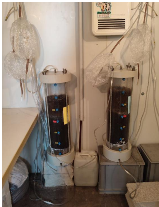
Figure 3.12 Columns under anaerobic conditions
