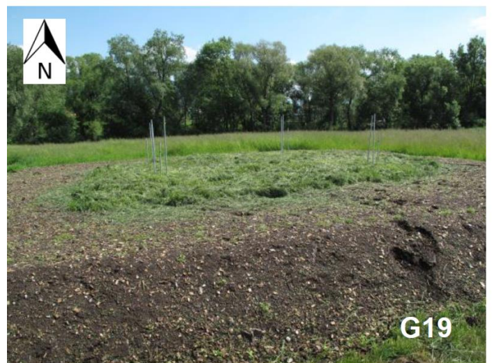
Figure 3.7 Photo of biowindow G19 after the enlargement (Hrad and Huber-Humer, 2015)
