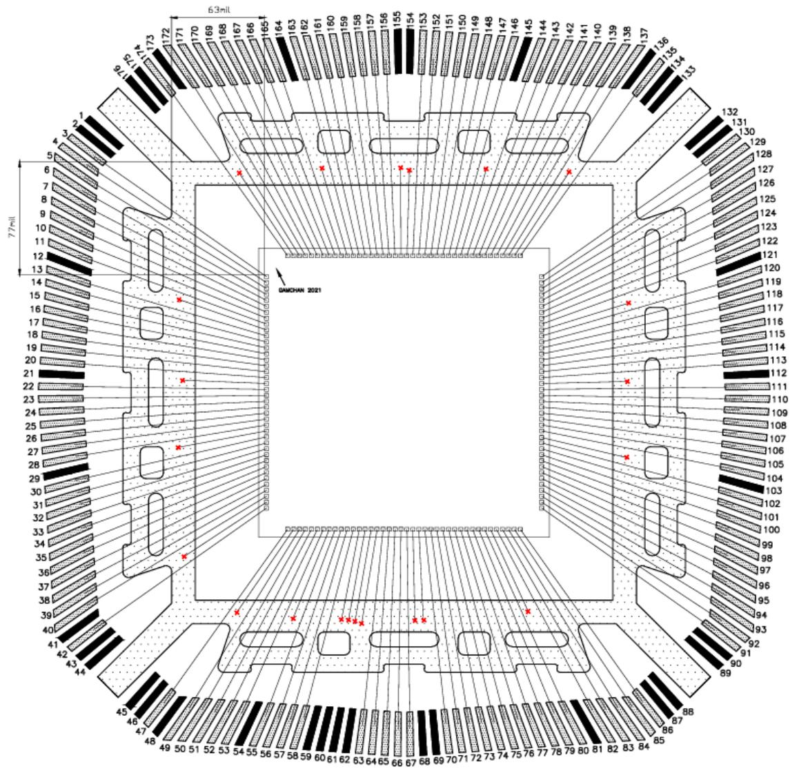
**Figure 2.17:** Bonding diagram of GAMCHAN
