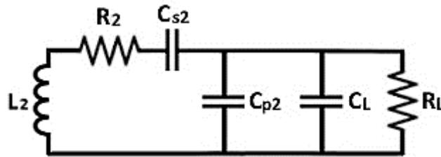
**Figure 3.22:** Complete output matching network
