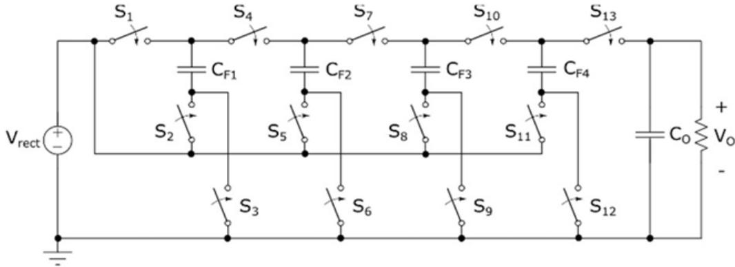
**Figure 2.9:** Simplified model of Dickson step-up converter with programmable conversion ratios  $n_i = (2, 3, 4, 5)$ .
