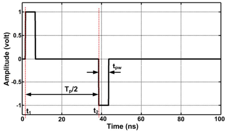
a) Narrow pulses generated at Tx for data bit “1”
