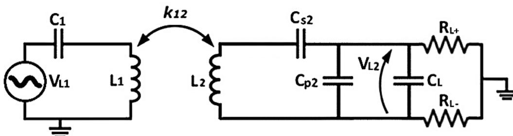
**Figure 4.2:** Setup scheme for the measurements of tab. 4.1
