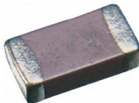
**Figure 3.11:** Generic SMD Multilayer Ceramic Capacitor
