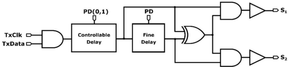
a) Pulse pattern generator diagram
