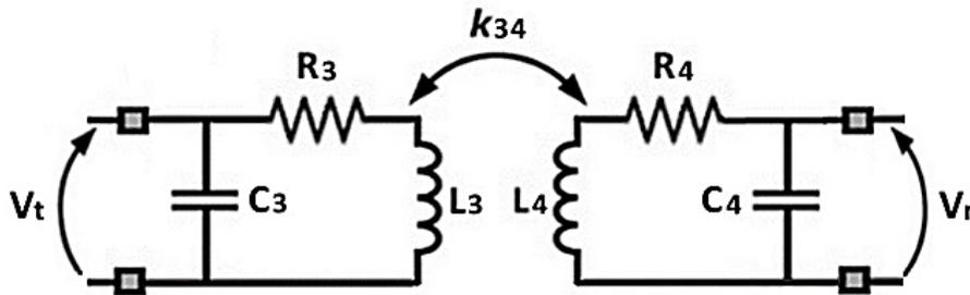
Figure 3.25: Data link equivalent circuit
