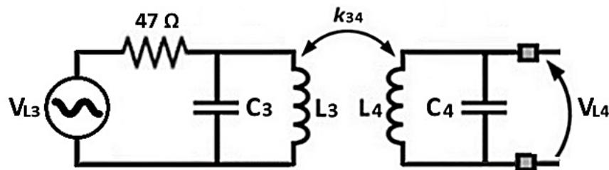
**Figure 4.3:** Setup scheme for the measurements of tab. 4.2
