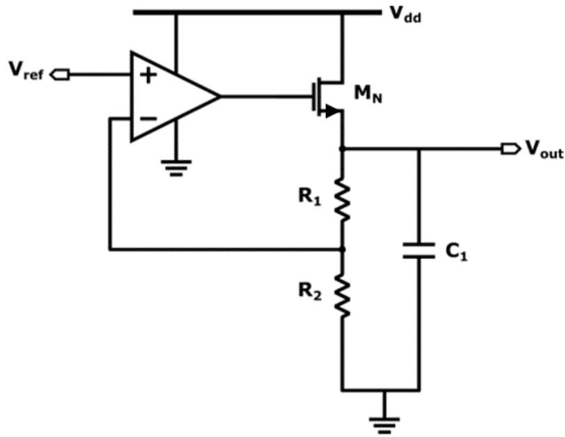
**Figure 2.10:** Low drop out voltage regulator (LDO)
