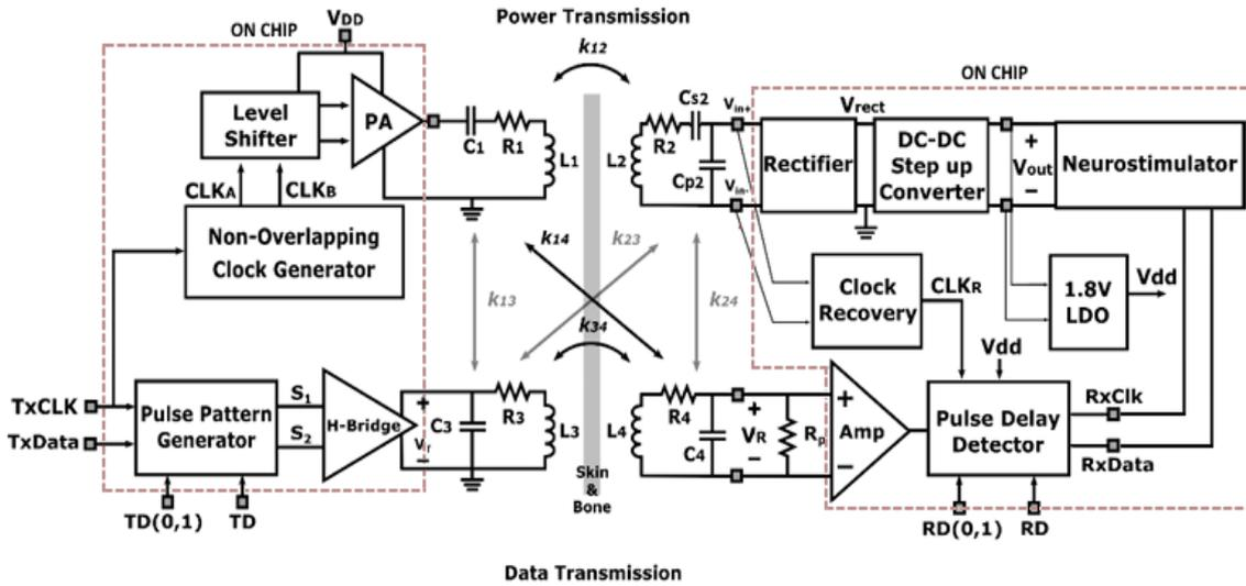
**Figure 2.3:** Block diagram of the full power and data transmission circuit system
