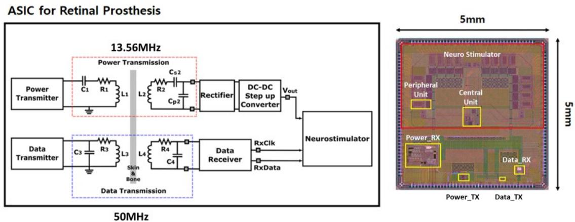
**Figure 2.2:** Inductive links for power and data
