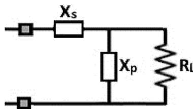
**Figure 3.21:** Generic scheme of the output matching network
