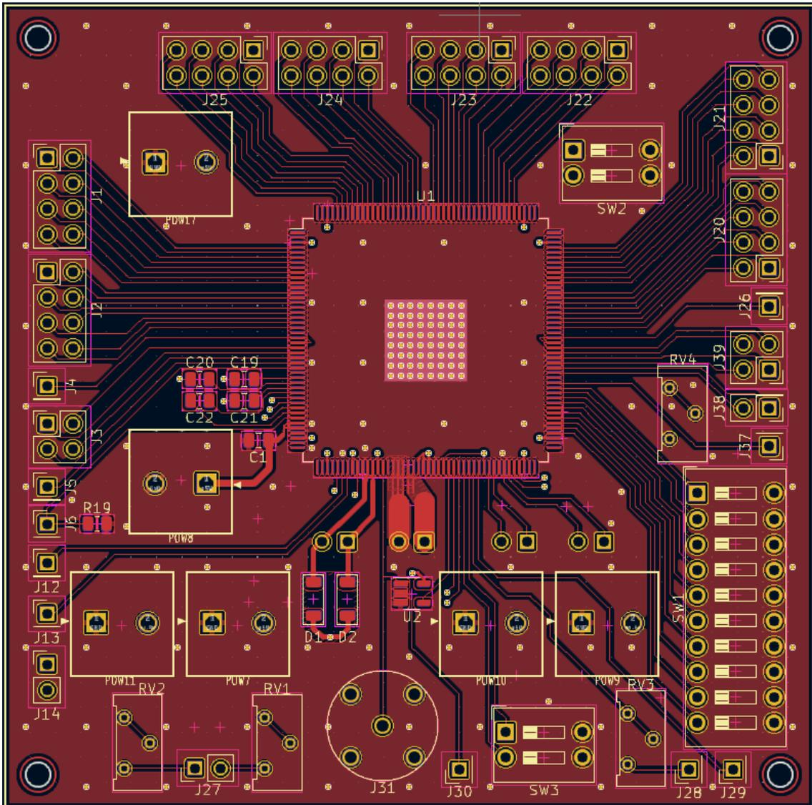
Figure 3.5: Front design scheme of the main PCB in Kicad
