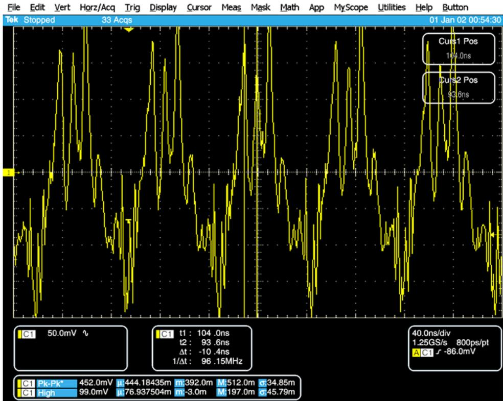
Figure 4.11: Single ended measurement of Ampin+/- with input data duty cycle 20%
