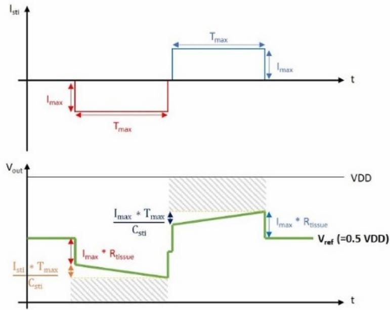
**Figure 2.20:** Current and output voltage change during stimulation
