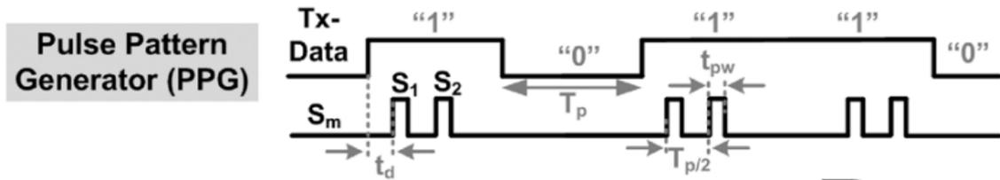
b) Pulse pattern generator operation
