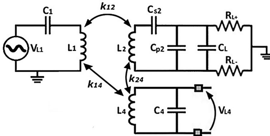
Figure 4.7: Setup scheme for measuring power carrier interference on  $L_4C_4$  data tank
