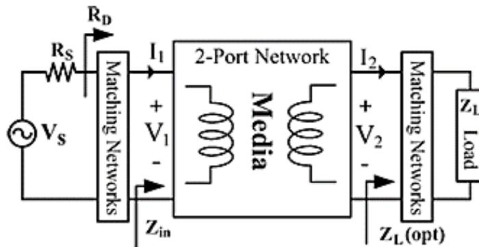
Figure 3.18: 2-Port network model for matching network calculation
