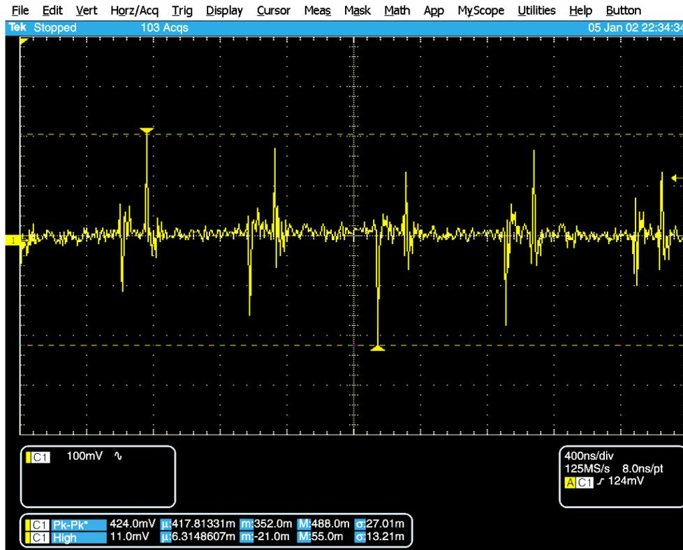
**Figure 4.8:** Single ended test measurement of L+/L- with CLK\_IN=5 V
