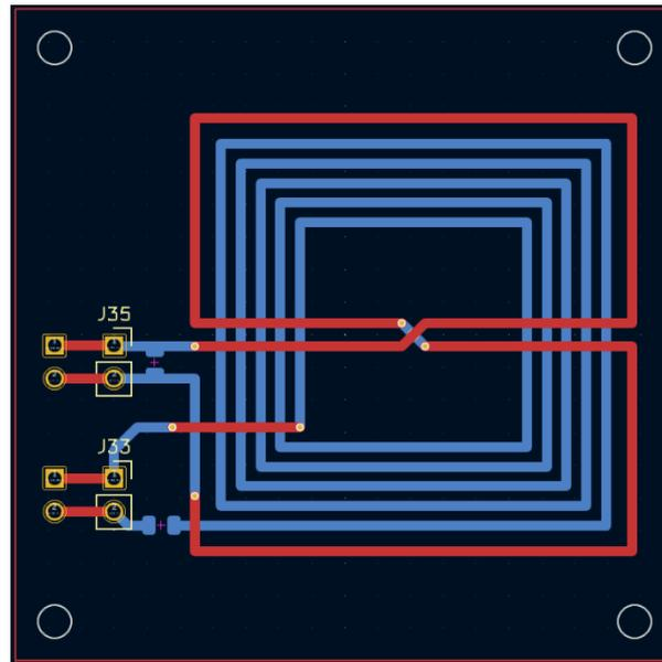
**Figure 3.28:** Tx printed inductors PCB ( $L_1$ ,  $L_3$ )
