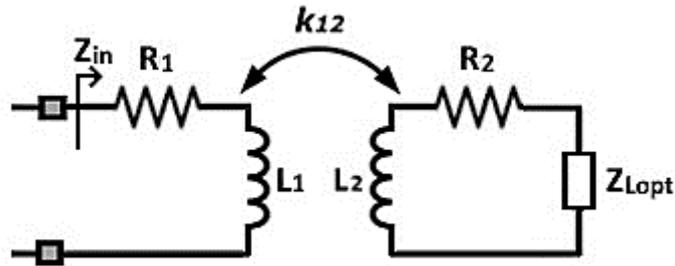
**Figure 3.23:** Input impedance seen at the input matching network
