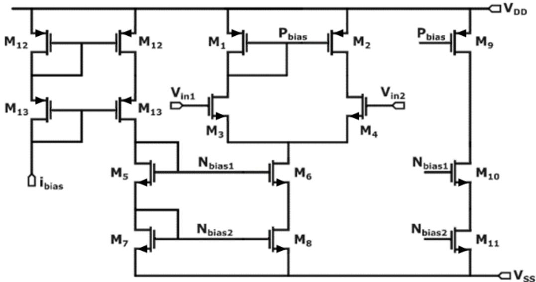
Figure 2.14: Data receiver amplifier
