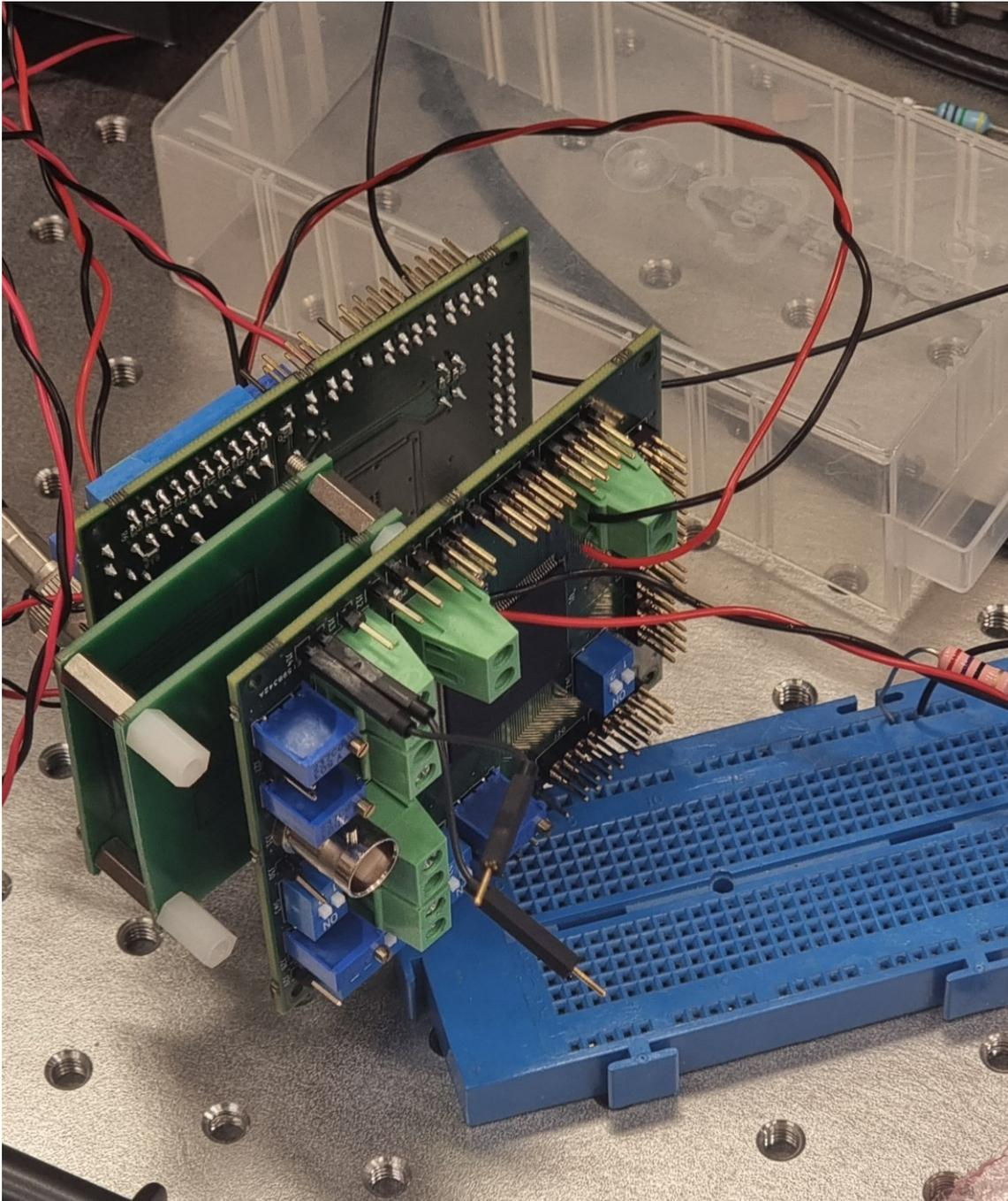
**Figure 4.4:** Lab setup for the measurement with both the Tx and Rx PCB
