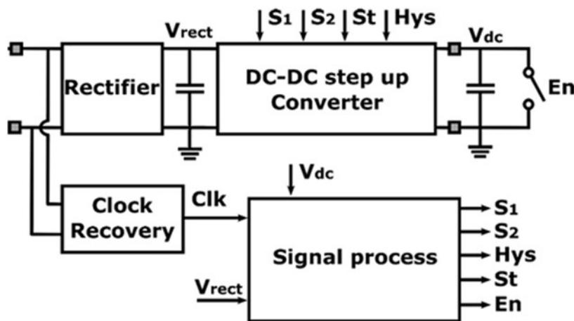
Figure 2.7: Power receiver block diagram
