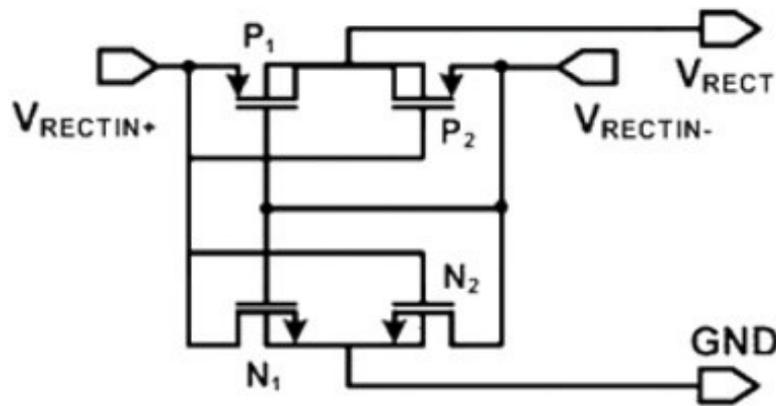
**Figure 2.8:** Diagram of the CMOS rectifier
