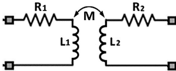
**Figure 3.19:** Simple model for inductive power transfer
