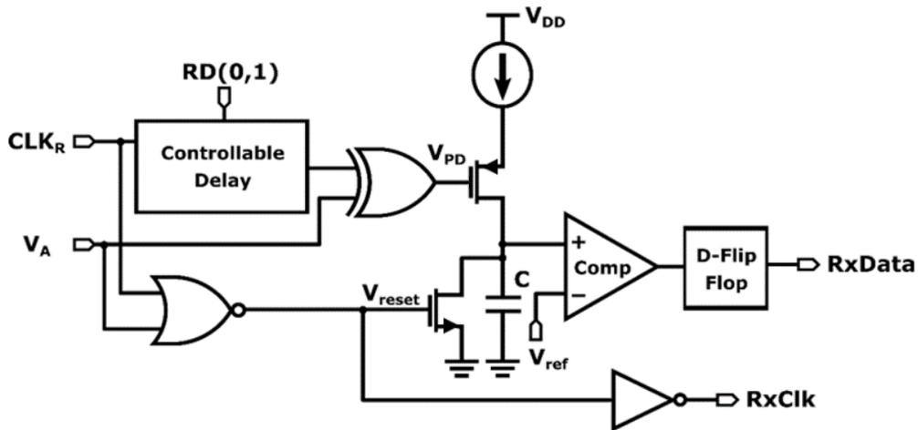
**Figure 2.15:** Pulse delay detector
