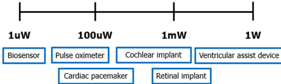
**Figure 2.1:** Different power requirements for IMDs
