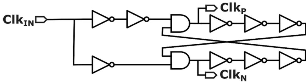
**Figure 2.5:** Non overlapping clock generator diagram
