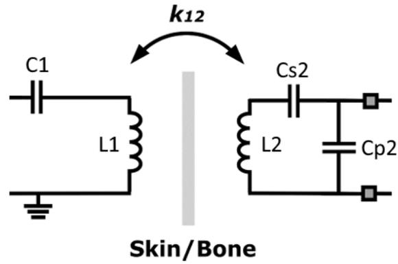
Figure 3.24: Power tank final scheme
