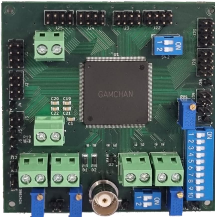
**Figure 3.17:** Fabricated main PCB with mounted components
