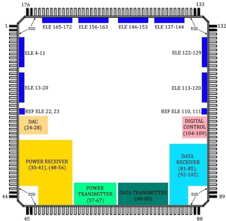
**Figure 2.18:** Different units of the chip
