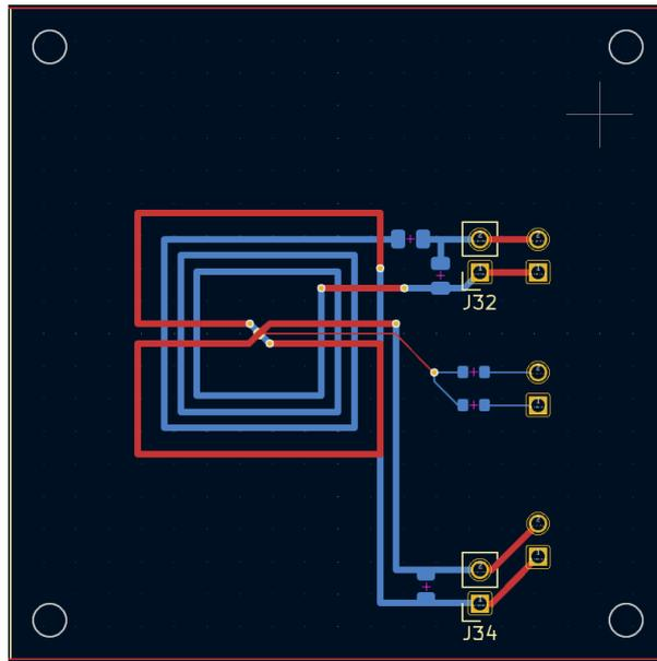
**Figure 3.29:** Rx printed inductors PCB ( $L_2$ ,  $L_4$ )
