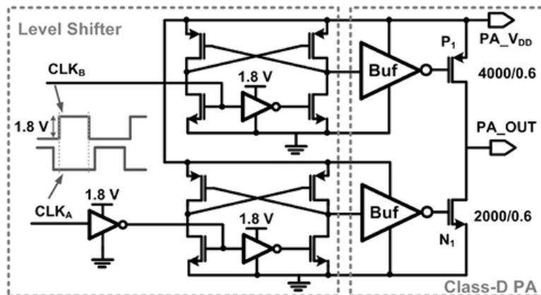
**Figure 2.6:** Level shifter, tapered buffer and output stage of PA
