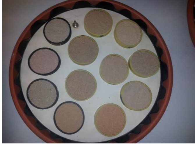
Figure 24. Soil samples in the pressure plate
