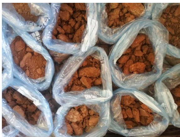
Figure 19. Preparation of the soil samples for chemical and physical analysis.
