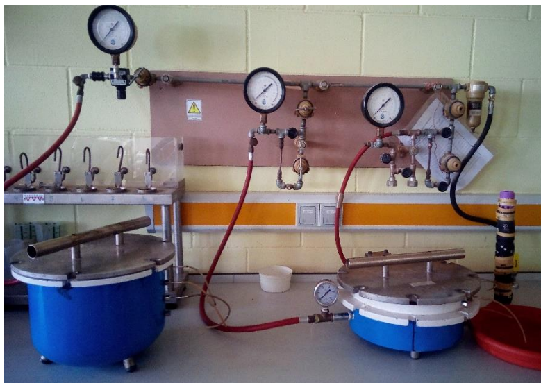
Figure 25. High-pressure equipment where Richard plates are collocated.
