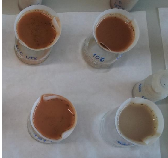
Figure 20. Filtration in the Electrical Conductivity analysis
