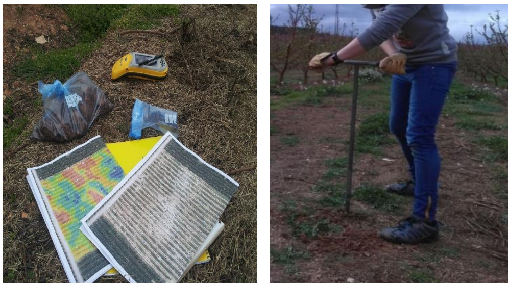
Figure 18. Right: Soil sampling in the study field by means of an auger hole. Left: Support material for soil sampling (GPS and ECa maps).
