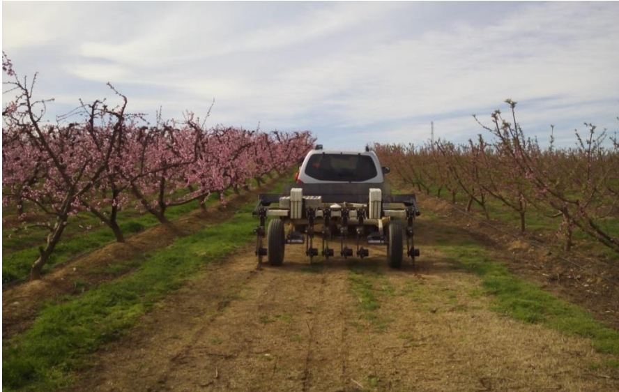
Figure 13. ECa survey conducted with Veris 3100 in the study field on 01/03/2016.
