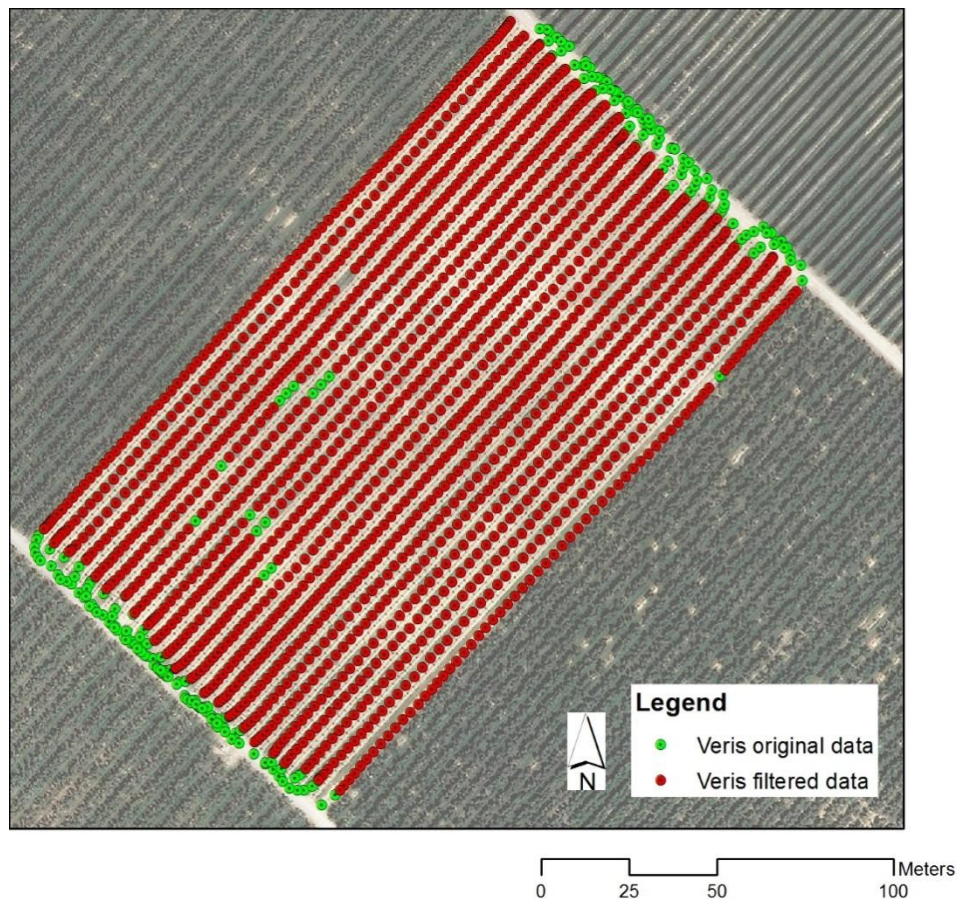
Figure 14. Veris 3100 original data acquired in the study field and data after filtering (turning line points and outliers). The visible green points were the ones that were removed by the filtering process. The red points were the data finally used in the interpolation.
