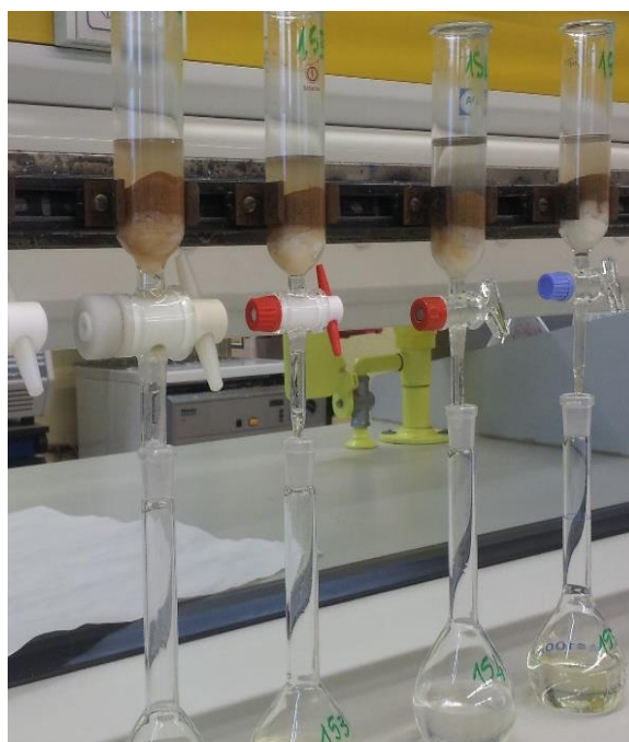
Figure 21. Percolation tubes with a filter of cotton wool-sand and soil sample
