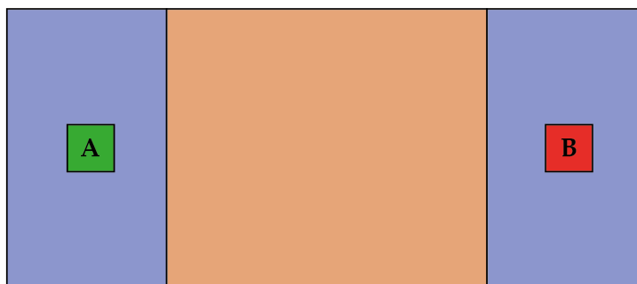
Figure 4.4: Uncoordinated bimanual setting. A \in S_L can be grasped only by e_L , B \in S_R can be grasped only by e_R
