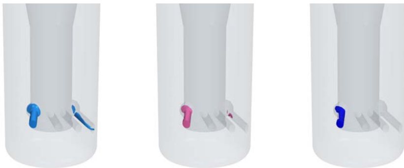
(a) 1% Volume fraction of vapor. (b) 5% Volume fraction of vapor. (c) 10% Volume fraction of vapor.
