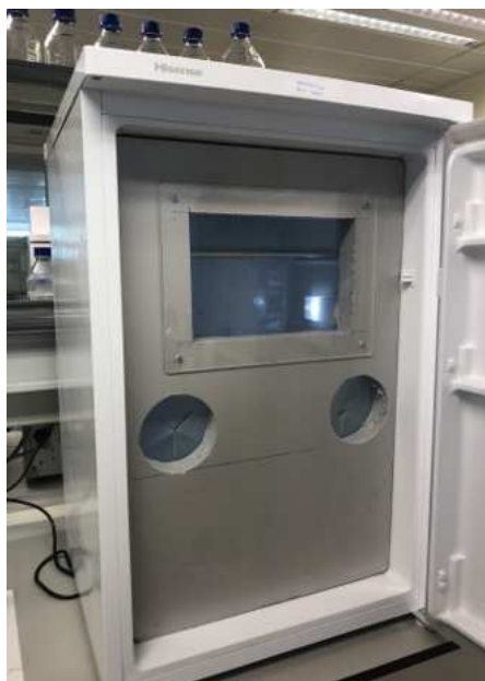
Figure 13: Mini fridge used for the synthesis of hydrogels at 4 °C
