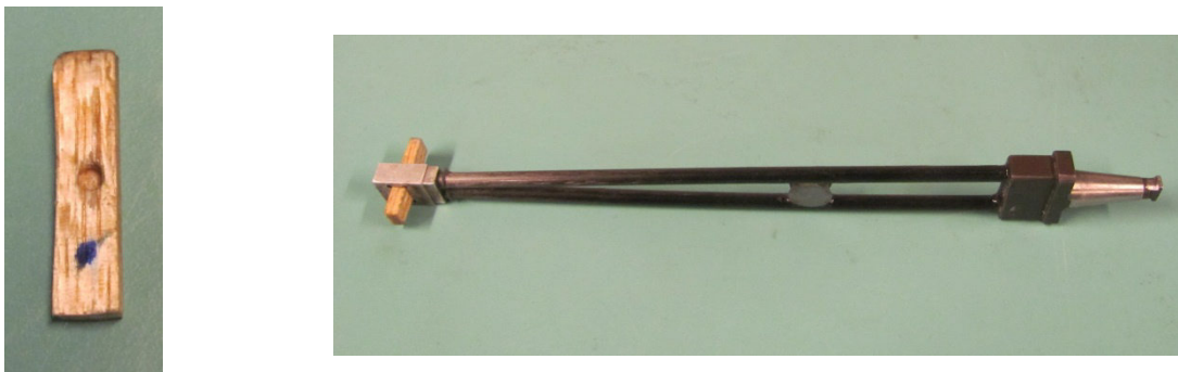
FIGURE 6.1. Image related to wood pad with its clamping system in the end of the polishing arm.
