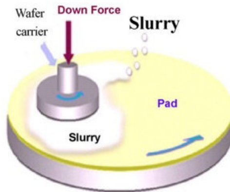
FIGURE2.3. General Chemical Mechanical Process employing rotational kinematic. [14].
