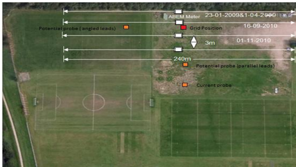
Figure 30 Soil resistivity measurement location at Llanrumney field site
