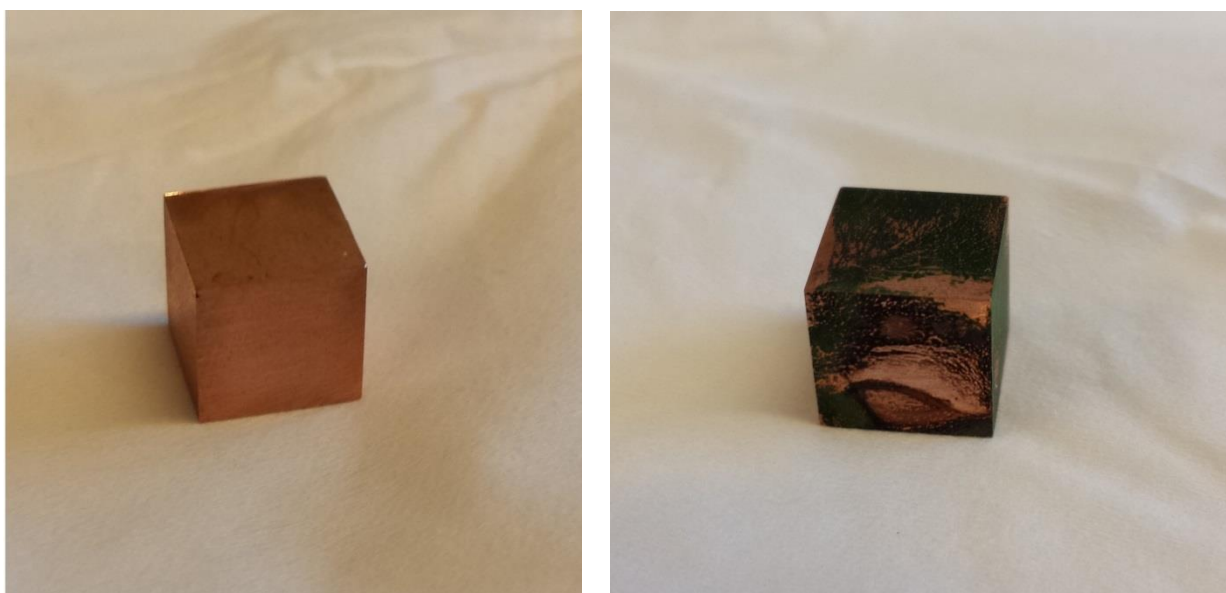
Figure 6.2 Depiction of the copper cube samples used in the overnight experiment, polished cube on the left and preoxidized cube on the right side.
