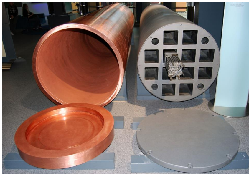
Figure 3. The ductile cast-iron insert in which are placed the twelve fuel assemblies.
