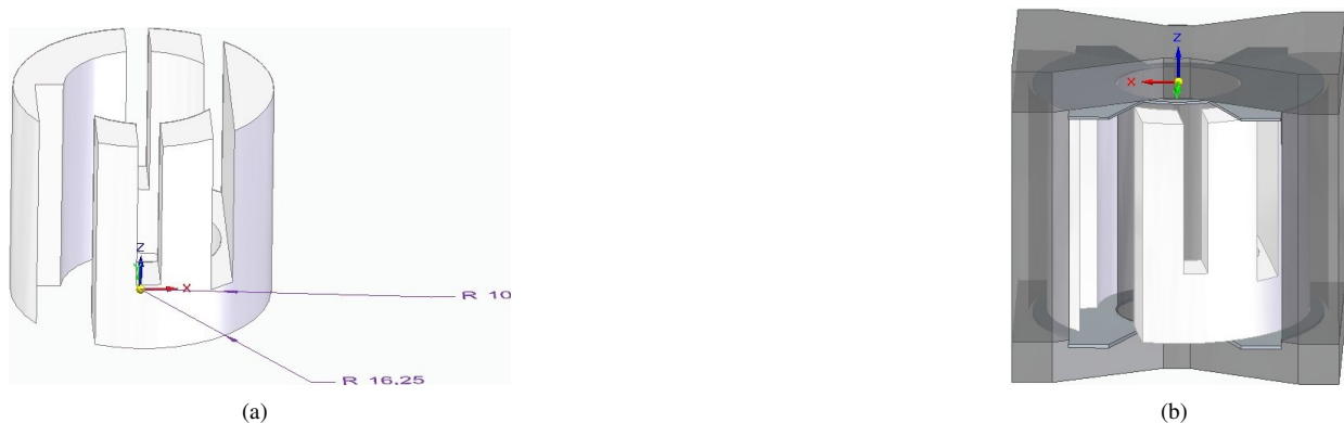
Figure 4.22: CAD design of the insulator and the total assembly.
