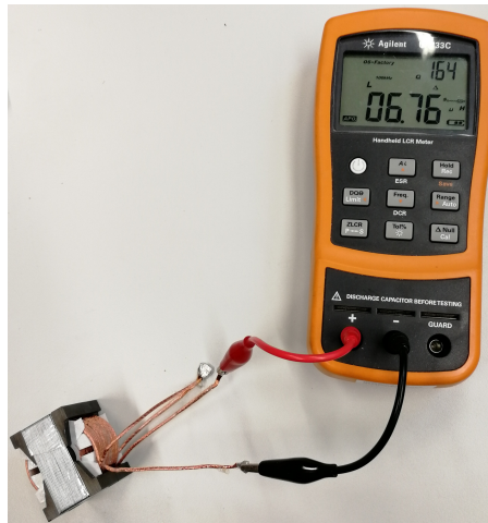
Figure 4.24: Leakage inductance measurement in the PQ4040.
