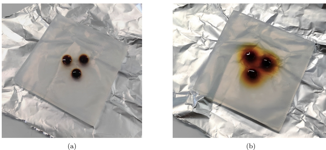
Figure 2.13: (a) Phantom with silver and agar solution inside the holes, dye is added for visualization reasons. (b) Same phantom after two hours. Diffusion process is clear.
