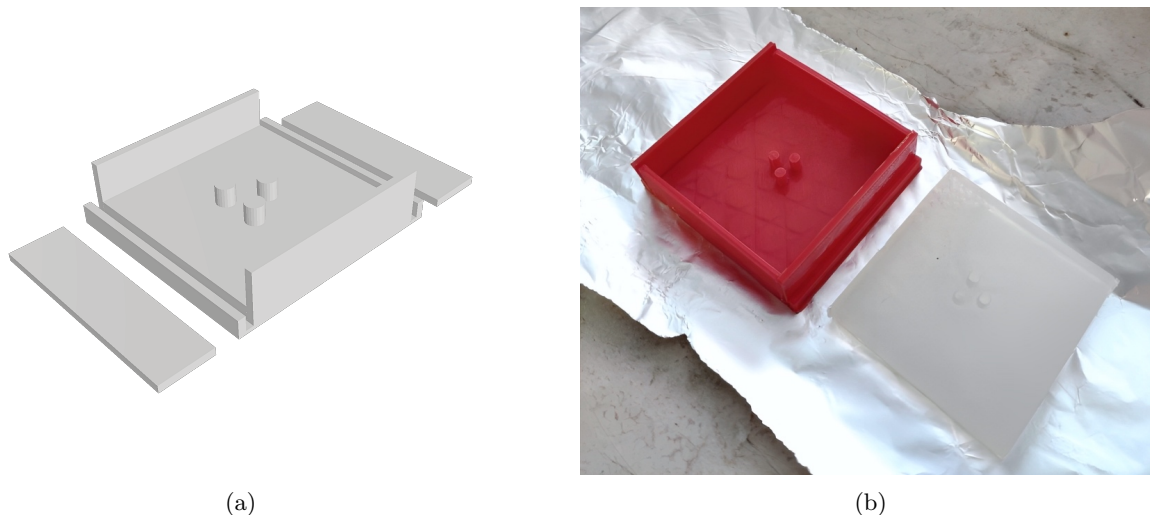
Figure 2.12: (a) Example of CAD project for a mold. (b) Picture of an agar phantom extracted from the mold.
