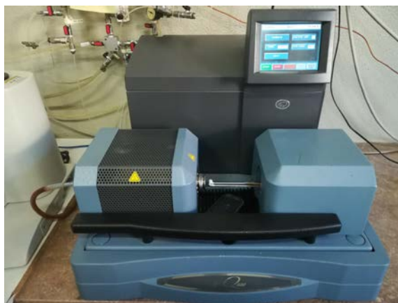
Figure 4.7: Thermo-gravimetric analysis apparatus, Q600 TA Instruments
