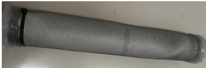
(b) Membrane rolled up on two plastic meshes.
