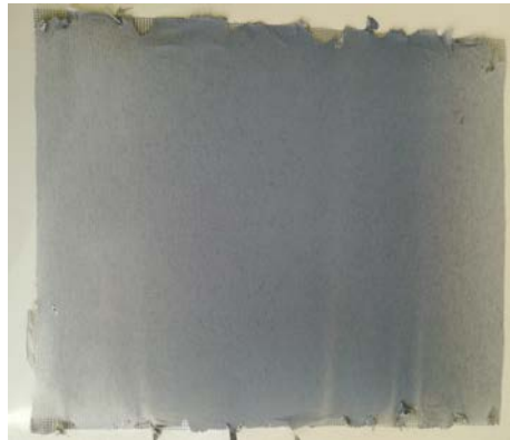
(a) Membrane deposited on a plastic mesh.
