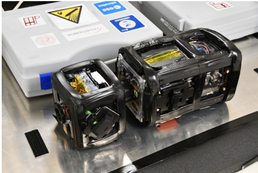
Figure 2.11: Chaser and Target in docked configuration
