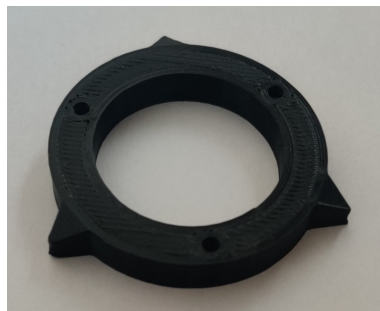
Figure 2.17: Release Structure - Centring component of the Release Interface
