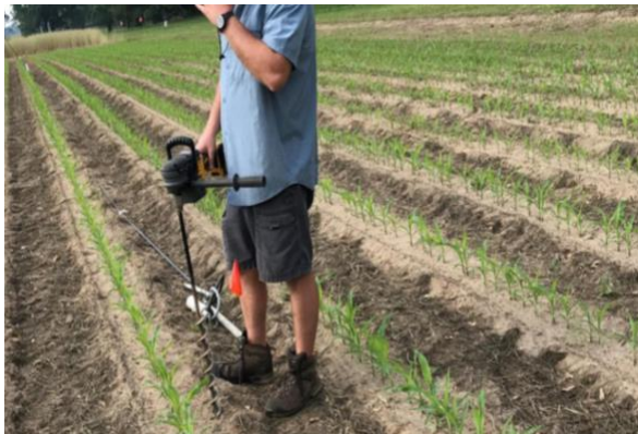
Figure 2-2. Installation by drilling a hole matching the geometry of the probe.
