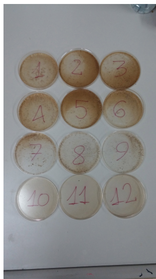
Figure 4.6: CNCs' samples: [1-2-3] from T1 (not proper CNCs), [4-5-6] from T2, [7-8-9] from T3 and [10-11-12] from T4.
