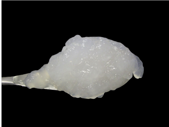
Figure 2.5: 2 % w/w microfibrillated cellulose aqueous suspension.
