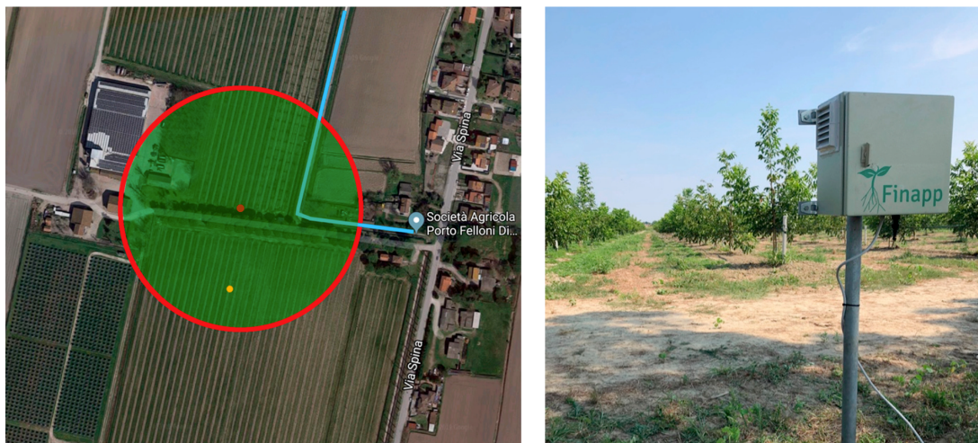
Figure 4.27: (Left) Field site (N 44.752756, E 12.134761), red point is where the Finapp probe was installed, the red circle is the footprint, the orange point represents where the five Sentek probes are installed at different depths, and the light blue line is the drainage canal. (Right) Picture of the installation.
