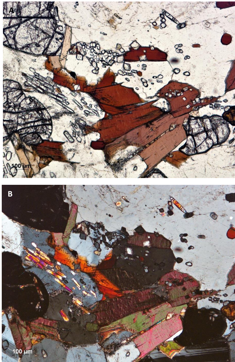
fig. 5.13. Sillimanite crystals included in plagioclase, garnet and quartz. A: plane polarized light; B: crossed polarizers.
