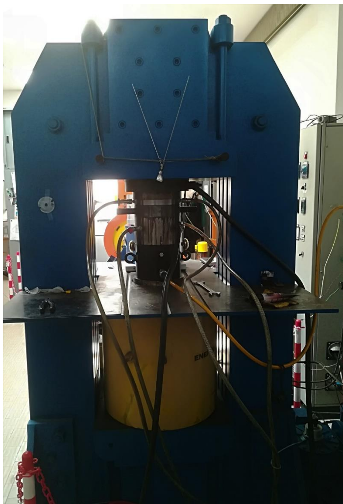
fig. 4.1. End-loaded piston cylinder at Department of Earth Sciences, University of Milan.
