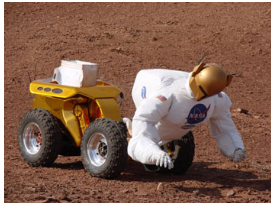
(d) Robonaut 1, developed by NASA, uses telepresence and has hands with fourteen degrees of freedom and use touch sensors at the tips of its fingers.
