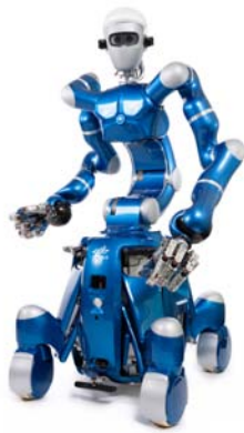
(c) Rollin' Justin, autonomous and programmable humanoid robot with two arms developed by the German Aerospace Center (DLR).
