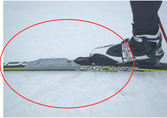
Fig 33: Detail of Xsens on the ski
