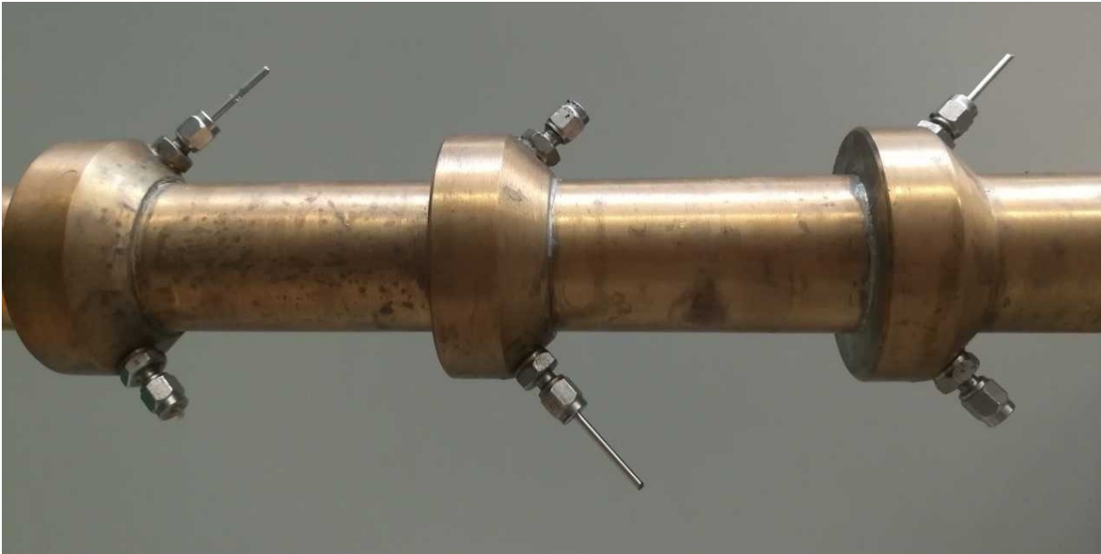
Figure 3.9: Disposition of the RTD sensors along the shell tube
