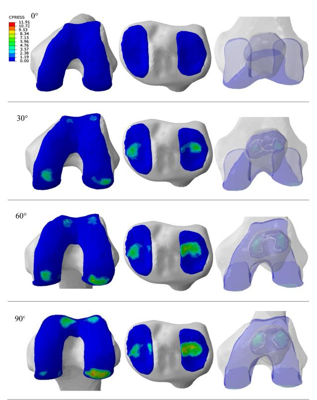
Table 4.5 - Contact pressure, measured in MPa, analyzed in femoral, tibial, and patellar cartilage during flexion for the patella alta model. In each cell, the left side represents the medial region, whereas the right side represents the lateral region. On the upper left side, contact pressure results are indicated in a legend with colors ranging from blue (0 MPa) to red (11.91 MPa).
