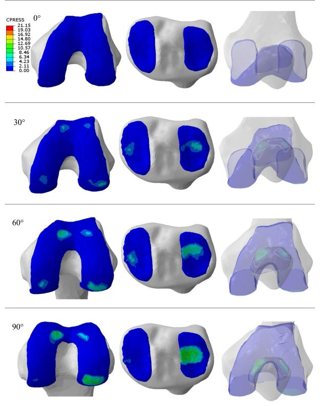
Table 4.6 - Contact pressure, measured in MPa, analyzed in femoral, tibial, and patellar cartilage during flexion for the patella baja model. In each cell, the left side represents the medial region, while the right side represents the lateral region. On the upper left side, the contact pressure results are indicated in a legend with colors from blue (0 MPa) to red (21.15 MPa).
