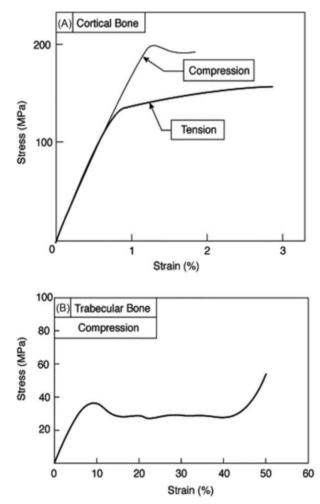
Figure 2.7 - Mechanical characteristics of cortical and trabecular bone. Common stress-strain curves representing cortical (A) and trabecular (B) bone samples subjected to compression or tension testing (Innocenti B. & Galbusera F., 2022).
