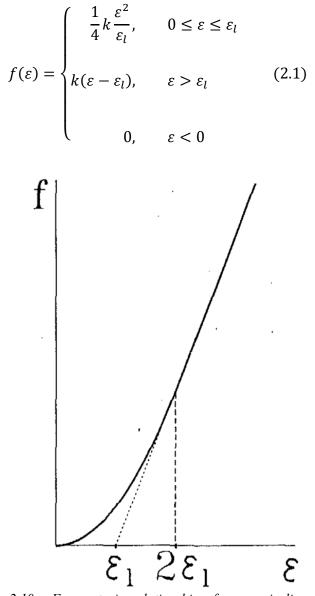
Figure 2.10 - Force–strain relationship of a generic ligament.  $\varepsilon_l$  is the threshold strain, which indicates the change from the toe to the linear regions (Blankevoort L., & Huiskes R., 1991).
