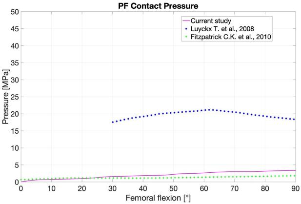
*Figure 4.16 - Comparison of patellofemoral contact pressure between the native model of the current study and the results obtained from the literature.*
