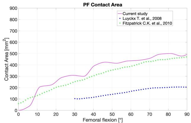
*Figure 4.14 - Comparison of total patellofemoral contact area between the native model of the current study and the results obtained from the literature.*
