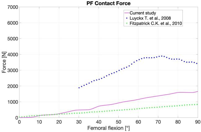
*Figure 4.15 - Comparison of patellofemoral total force due to contact pressure between the native model of the current study and the results obtained from the literature.*
