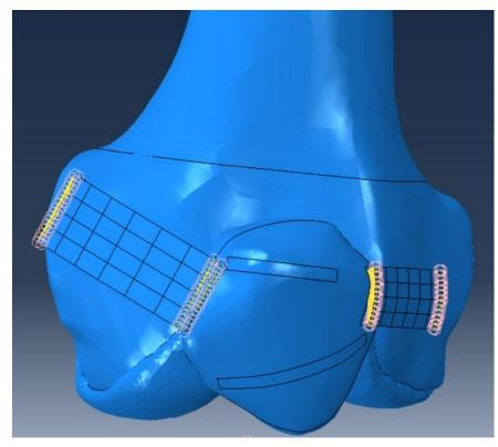
*Figure 3.10 - Coupling between the bone components and the MPFL and LR. Highlighted in pink are the nodes used for the constraint.*
