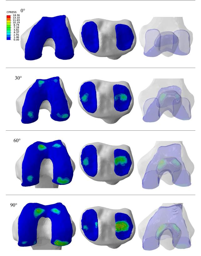
Table 4.4 - Contact pressure, measured in MPa, analysed in femoral, tibial, and patellar cartilage during flexion for the native knee model. In each cell, the left side represents the medial region, whereas the right side represents the lateral region. On the upper left side, contact pressure results are indicated in a legend with colors from blue (0 MPa) to red (14.56 MPa).
