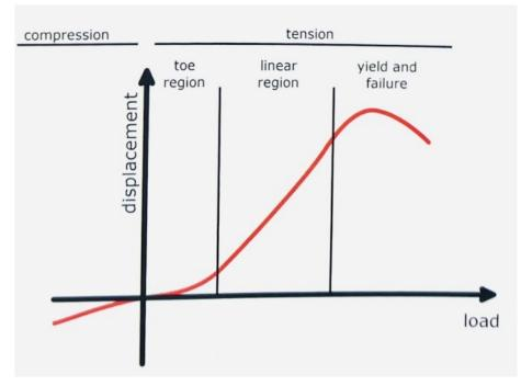
Figure 2.9 - An illustrative uniaxial load-displacement graph of ligaments and tendons, demonstrating the toe region, the linear region, and the segments where yield and failure occur (Innocenti B. & Galbusera F., 2022).
