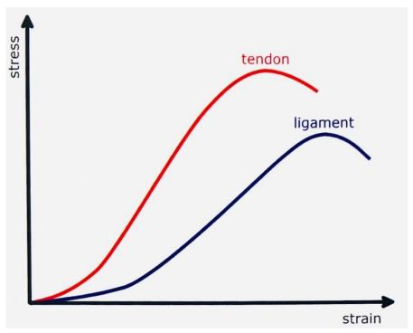
*Figure 2.8 - The unique stress-strain profiles of tendons and ligaments emphasize the higher stiffness and strength exhibited by tendons (Innocenti B. & Galbusera F., 2022*
