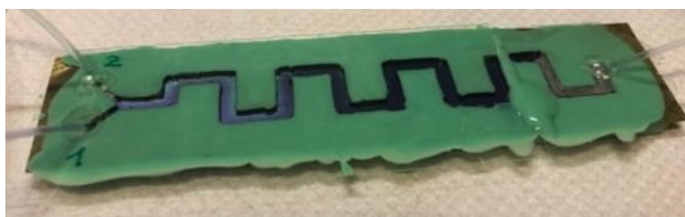
Figure 2.4.10: second iteration of the chip, photo taken right after running the experiment with the dyes.
