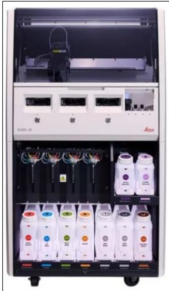
FIGURA 15: BOND RX Automated IHC (Leica biosystem, Wetzlar, Germany) con le taniche contenenti i solventi ( epitope retrieval 1 e 2, dewax solution, DI water, wash buffer, Alcohol ) ed i rifiuti ( bulk waste e hazardous waste ).
