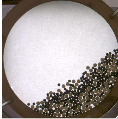
Figure 3.78. Example of image used for the evaluation of the Dynamic Angle of Repose for the mixtures of 8 mm spheres and 6 mm spheres.
