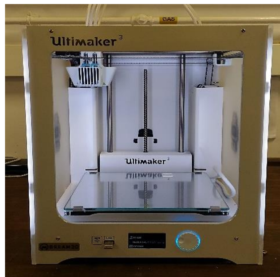
Figure 2.5. Ultimaker 3D printer used to print some of the non-spherical particles.
