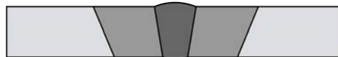
Figure 1.1: The cross-section of a welded butt joint. The darkest grey represents the weld, the medium grey the heat-affected zone and the lightest grey the base material.
