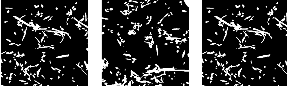
Figure 3.4: Representation of three sections of the solid obtained by X-ray tomography and used by the Matlab code to obtain the peridynamic solid.
