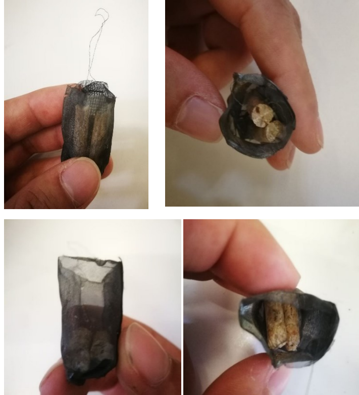
Figure 76 Pellets inside the basket in vertical and horizontal positions
