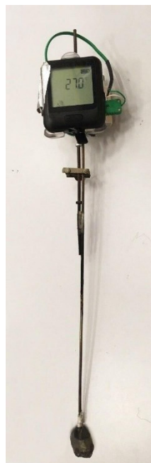
Figure 25 Temperature data logger
