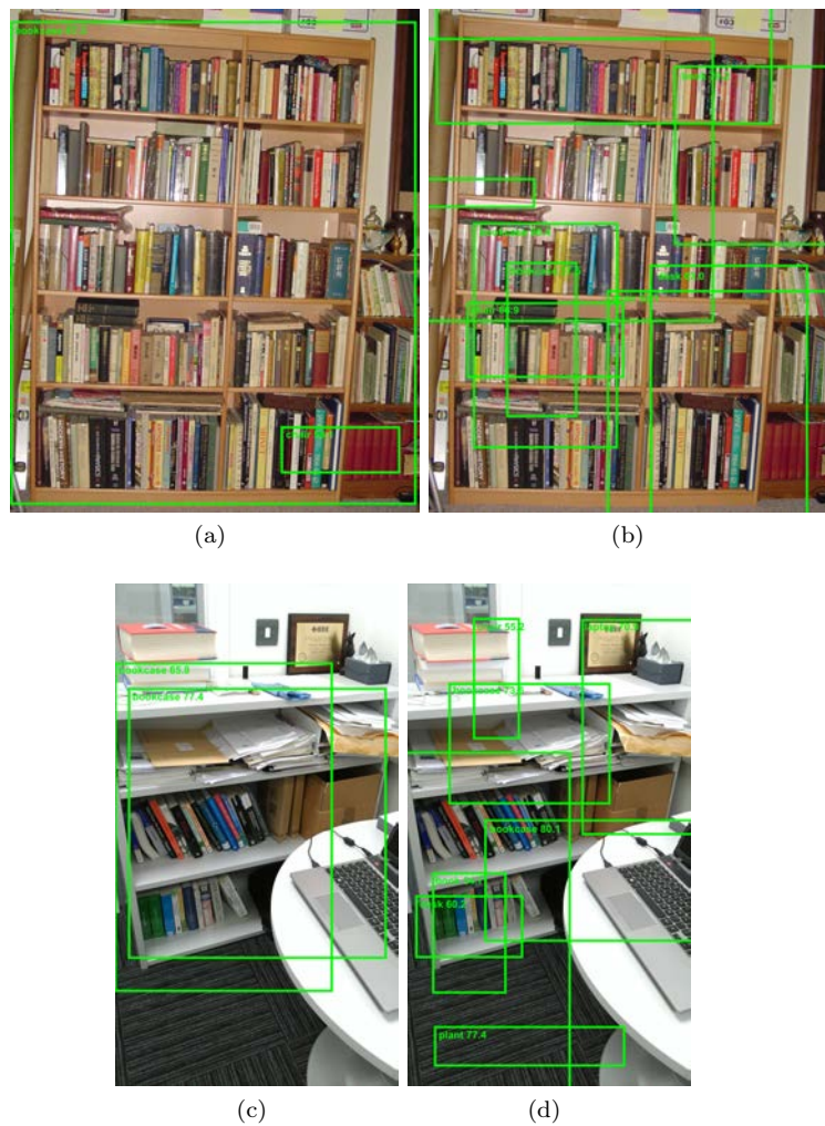
Figure 4.7: Prediction examples of SSD-Lite (a)(c) and Tiny-DSOD (b)(d) on OpenImage test set (a)(b) and Office test set (c)(d). A confidence threshold of 50% is used in these predictions.
