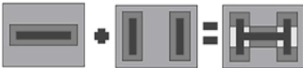
Figure 1.21. Assumed stress distribution under base plates in T-Stub method (CWE Journal Stress distribution)
