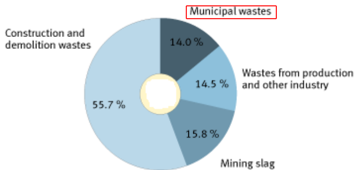
Figure 6.6: General waste composition in Germany (Destatis, 2014)
