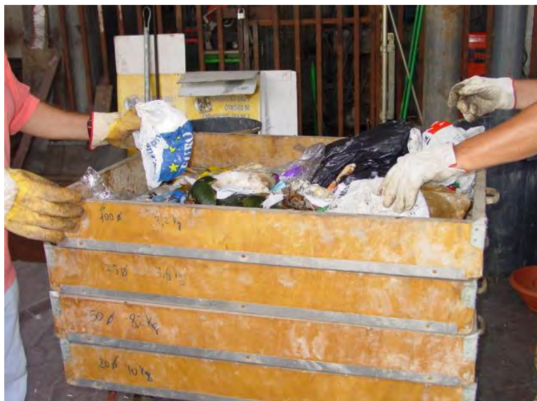
Figure 6.14: Different overlapped sieves, which are manually moved, allowing the smaller waste fraction to reach the bottom layers (Cossu, 2012)
