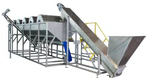
Figure 10.10: Swim-sink separator (Ctsmachinery, 2015)
