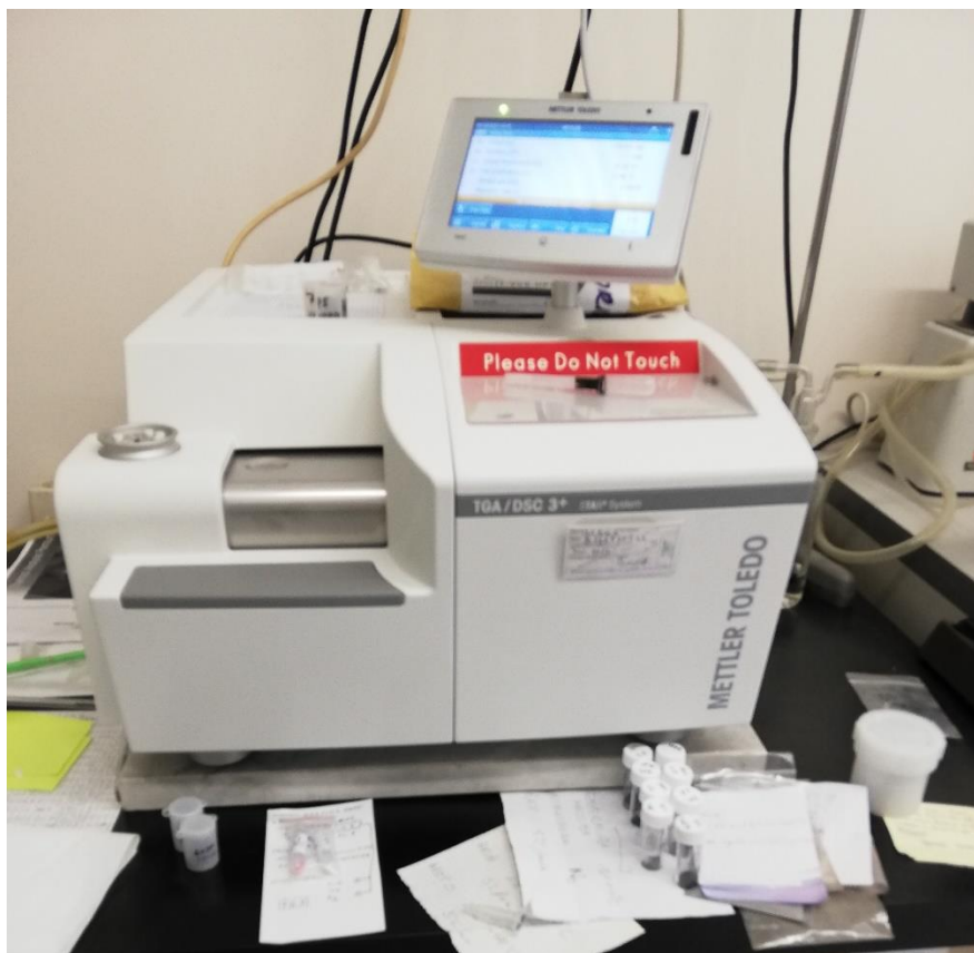
Figure 3.5. DSC/TG machine by Mettler Toledo.
