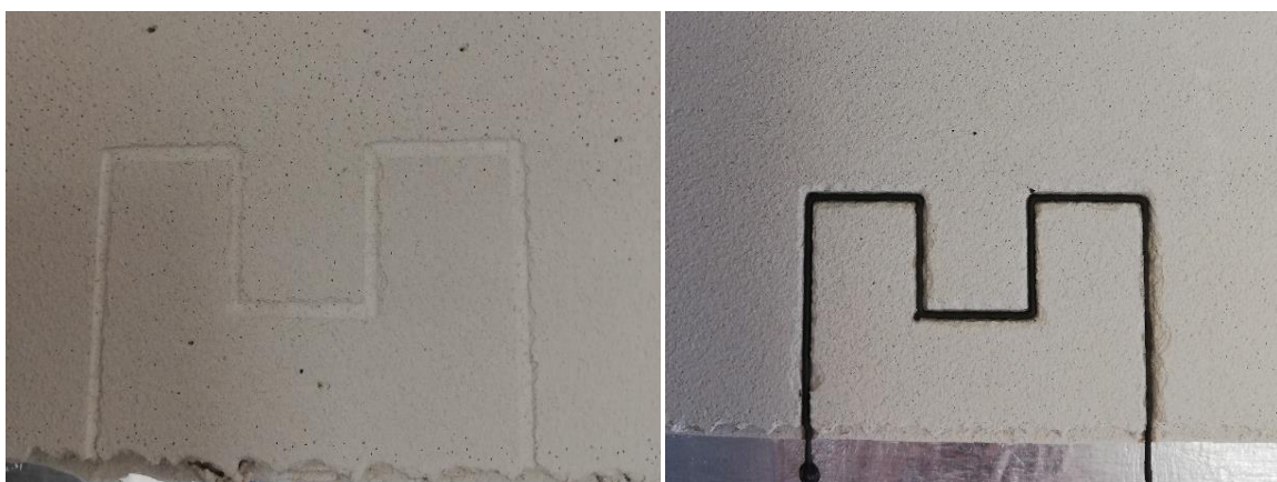
Figure 3.11. Example of a simple drilling and ink printing path.
