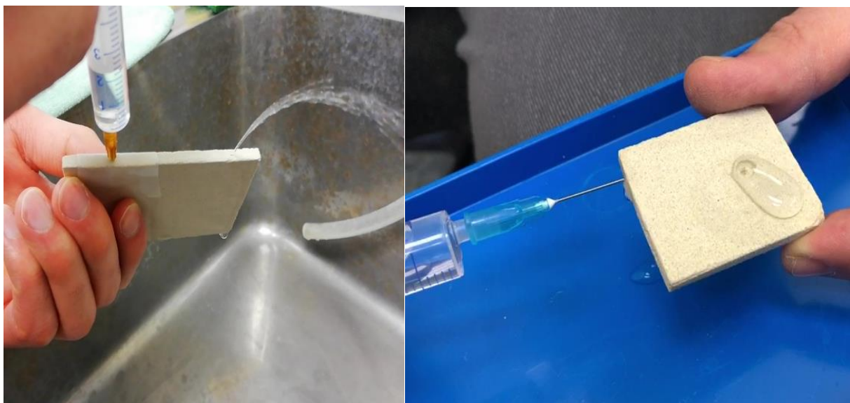
Figure 4.29. Demonstration tests of the fluid flow inside the built channels.
