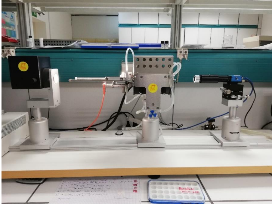
Figure 3.3. Hot stage microscopy - Hesse-Instruments, Osterode am Harz.
