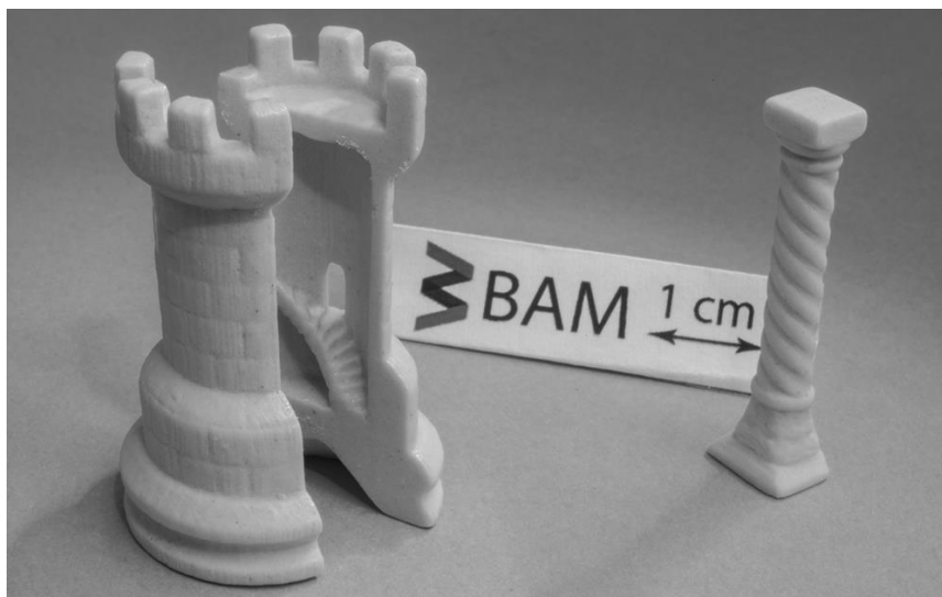
Figure 2.10. Example of LSD-printed porcelain samples 23 .
