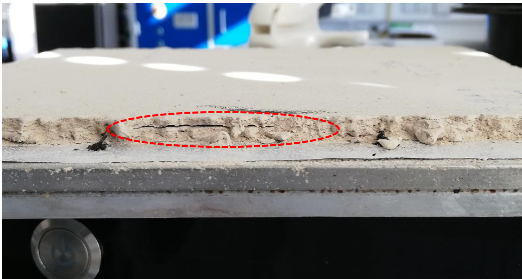
Figure 4.15. Lateral view of the green LSD part, delamination is visible over the channel.
