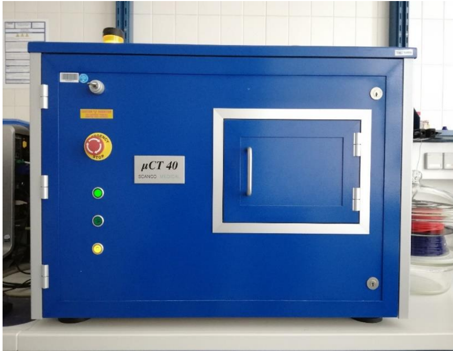
Figure 3.13. Micro computed tomography machine by Scanco Medical used for the analysis.
