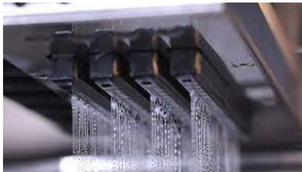
Fig. 9. An example of binder jetting process.
