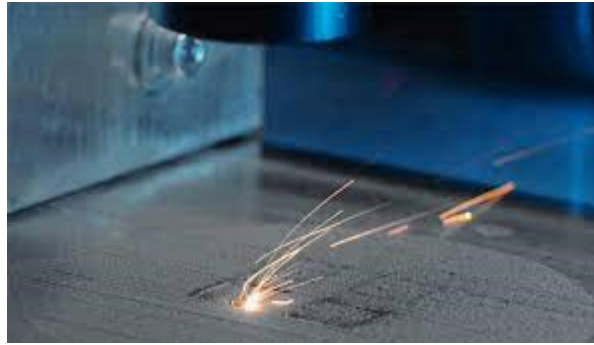
Fig. 2. An example of powder bed fusion process
