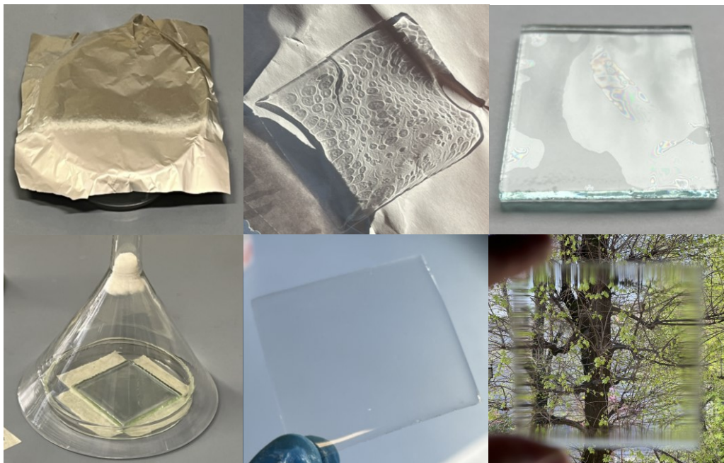
Figure 3.12. Pictures of stages and issues of the pure PMMA film making: the upper line attested the superficial imperfections and self-detachment of the film when adopting the aluminum-sheet-coverage method; in the lower line the improved method with a cottoned funnel cover, the resulting detached film and the visibility through it are shown.
