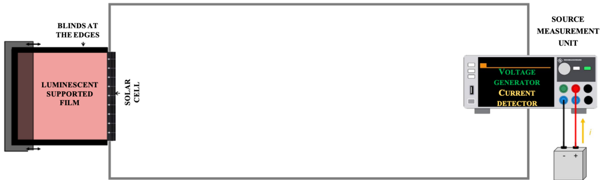
Figure 5.1. Schematics of the employed electronic circuit for measuring the performances of the developed LSCs films. The label V specifies the voltmeter, A the amperemeter and SMU designates the source meter unit.
