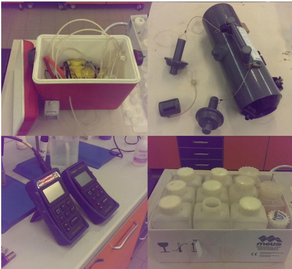
Figure 2.6 From top left to bottom right: the vacuum pump used for sampling, the Niskin bottle and the "messaggero" (between the two caps), the two WTW multiparametric probes, the 1000 mL bottles used to contain the samples.
