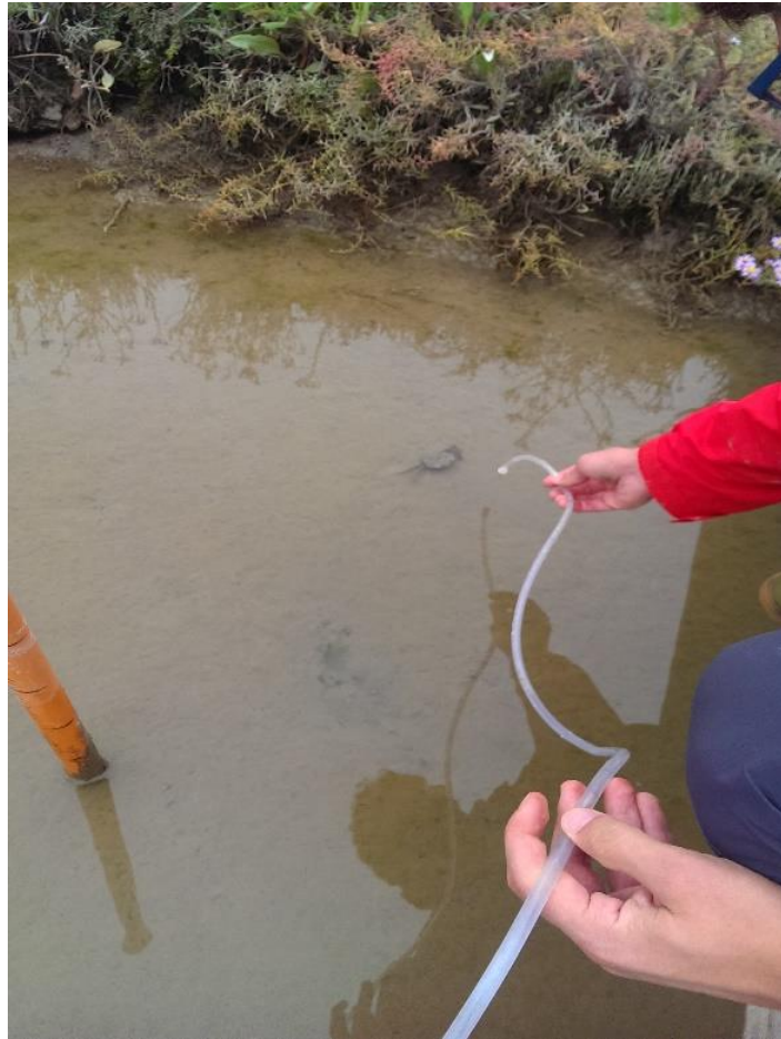
Figure 2.7 Sampling in the marsh creek using the vacuum pump and the pierced plastic tube.
