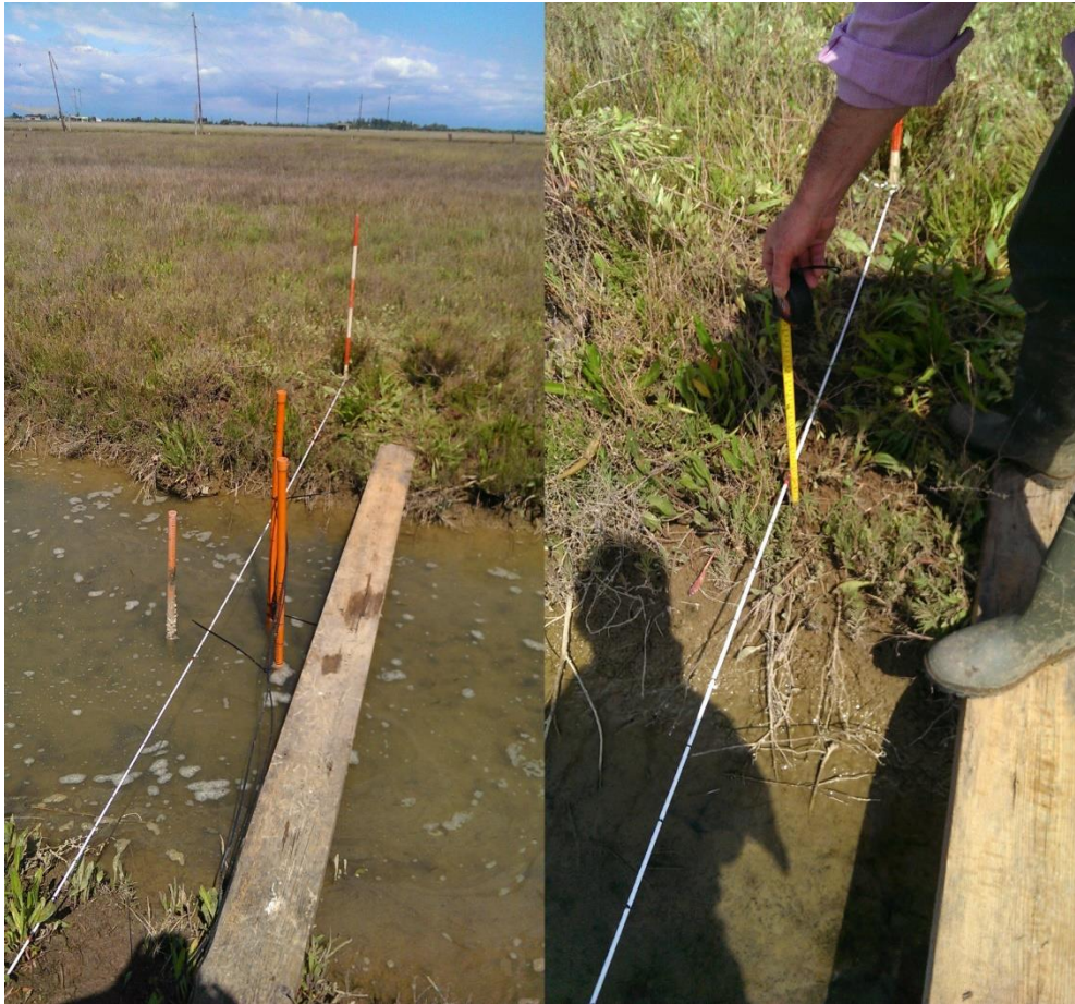
Figure 2.8 On the left, the positioning of the rope perpendicular to the creek for the cross section analysis; on the right, vertical measurements are taken.
