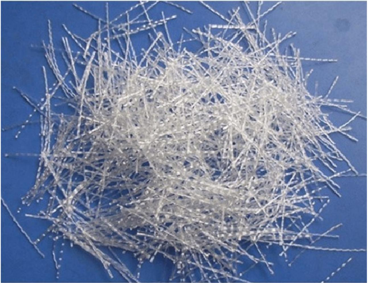
Figura 15 Fibre in polipropilene
