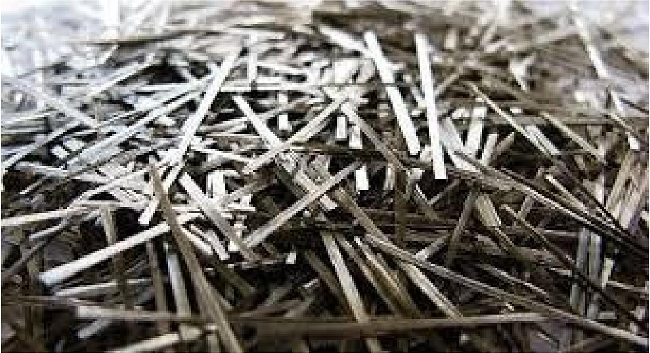
*Figura 11 Fibre in basalto*
