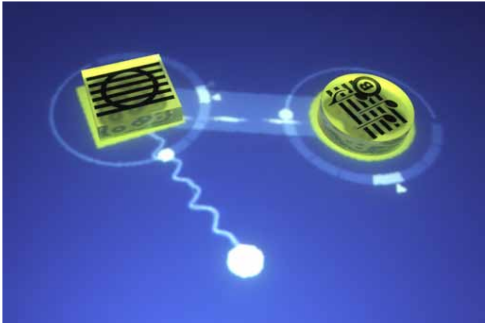
Figure 1.6. Current implementation of Sequencer in the Reactable. Here we see the Sequencer sending notes to a “plucked strings synthesizer”. Around the Sequencer we see an upper half ring for volume control and a lower half ring for melodies that must be stored in advance.
