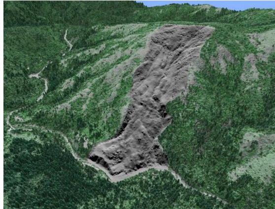
Figure 1.5 Rendered LiDAR image illustrating deep seated landslide underneath vegetative cover. South Fork Eel River confluence with Tenmile Creek. Image: Collin Bode, 2010. LiDAR: 2004, NCALM. ( http://criticalzone.org )
