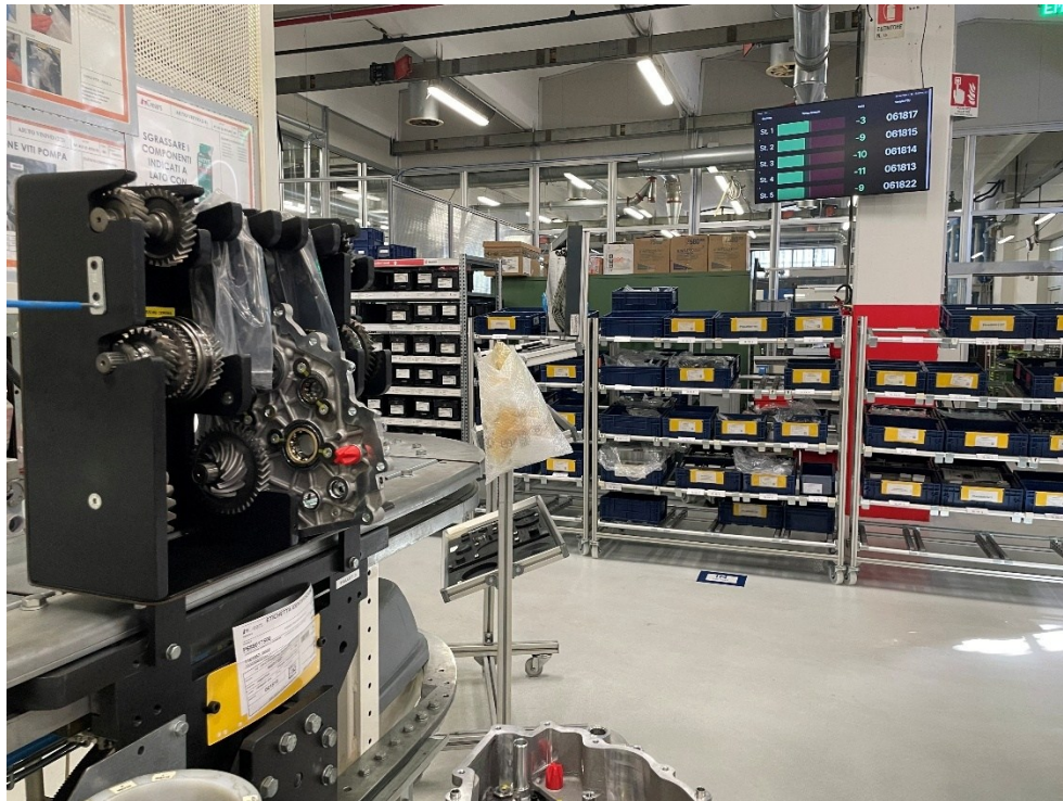
Figure 5 - The assembling station of transmissions with enabled monitor production system
