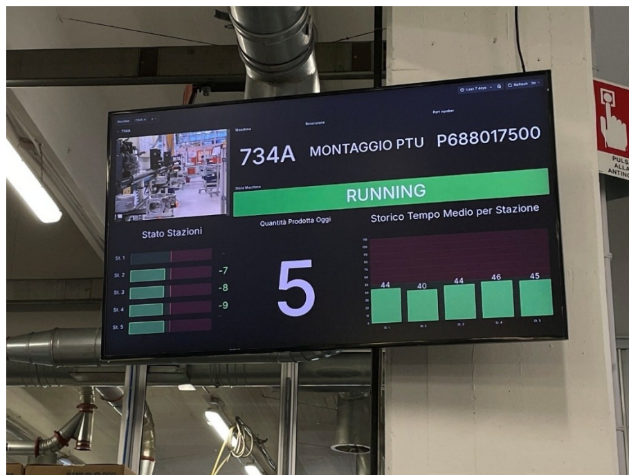
Figure 6 - The screen of the monitoring system with established cycle time and number of units to be assembled during the working day
